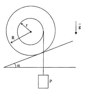
A stepped block whose radii are r and R, and the force of gravity is G, is located on an unsmooth inclined plane. A thread is wound on the inner step of the block; a load is suspended to the end of the thread. The coefficient of friction of adhesion between the block and the plane is f.
