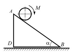
The triangle prism of mass 2m is placed on the smooth horizontal plane. An angle at a base of the prism is  $\alpha$ . On the edge AB of the prism a solid homogeneous cylinder of mass m and radius r rolls under the action of moment *M*. The friction coefficient between the cylinder and the prism is *f*.
