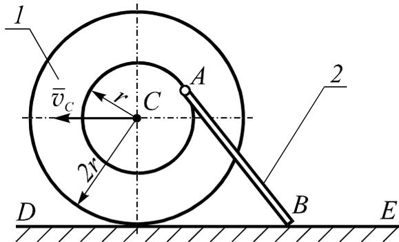
The stepped wheel 1 has radii  $r$  and  $2r$  and rolls along the plane  $DE$  without slipping. The center of the wheel  $C$  has a constant velocity  $v_C$ . At the point  $A$  the rod 2 is connected to the wheel by the hinge. The length of the rod 2 is equal to  $3r$ . The end  $B$  of the rod slides along  $DE$ .
