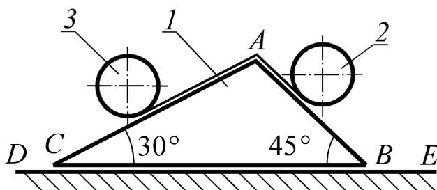
The triangular prism 1 of mass  $2m$  is on a rough horizontal plane  $DE$ . The prism has smooth facets  $AB$  и  $AC$  and it can slip along the plane. Homogeneous solid cylinders 2 and 3 each of mass  $m$  are on the facets  $AB$  and  $AC$  correspondingly. The cylinders are connected by an inextensible weightless thread.
