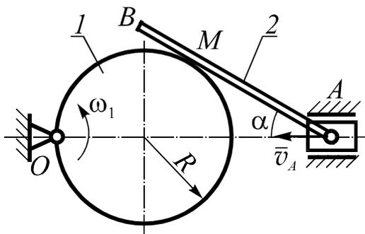
The cam 1 of radius  $R = 4\sqrt{3}$  cm rotates with the constant angular velocity  $\omega_1 = 2$  rad/s and sets in motion the rod 2 resting on it at the point  $M$ . At the point  $A$  the rod is connected to the slider. The slider moves along the horizontal direction with the constant velocity equal to 3 cm/s.
