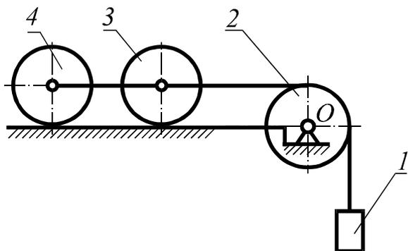
The load 1 is suspended by a weightless thread which is thrown through the block 2. The block rotates around a fixed horizontal axis  $O$ . It sets in motion the rollers 3 and 4 on a horizontal plane. The masses of body 2, 3 and 4 are the same and are equal to  $m$  each. The pulley 2 and the roller 3 are the solid homogeneous discs, the mass of roll 4 is evenly distributed over its rim. Coefficient of friction between the rollers and the surface  $f < 1$ .
