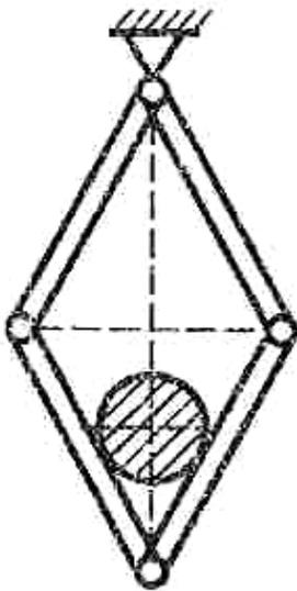
Four identical homogeneous rods of weight  $G$  and length  $l$  each are pivotally connected to each other and form rhombus. The upper hinge of the rhombus is connected to the motionless support. A homogeneous cylinder of weight  $P$  is inside the rhombus in the equilibrium if the angle between the upper rods of the rhombus is equal to  $2\alpha$ .
